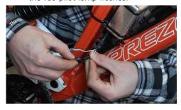
4.0 Connect the USB adapter to the PC USB port and to the BDL Module.
