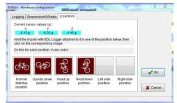
Place the bike in each of the 6 positions and at each position click on the correct image to set the sensor.
