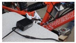
3.0 Connect battery power to the BDL Module. When the unit is powered, the red pilot lamp flashes.
