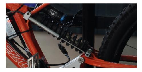
As was the case with the front travel sensor, the mounting must be such that the rod is parallel to the shock and full suspension travel is accommodated by the sensor.
