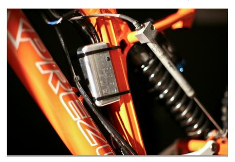
To get smoother G force readings with less spiky noise, it is suggested to have some kind of damping between the frame and module. A good way to achieve that is to attach rubber tubes to the BDL module, then attach those tubes to the frame.
