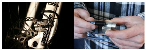
Put electrical tape where you want to install the bracket on the fork. Depending on your fork diameter, use one or more layers of tape such that the bracket adapts comfortably to the fork. 3M Dual Lock Tape can also be used if preferred.
